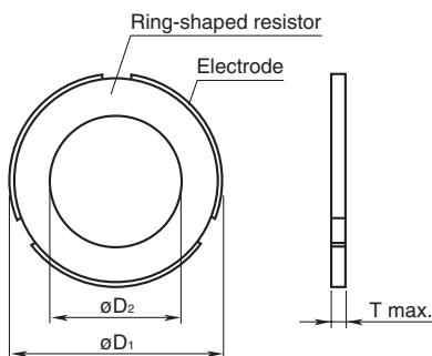
**SIDE SURFACE ELECTRODE TYPE(6-ELECTRODE)**
