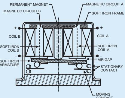
When latching relays are installed in equipment, the latch and reset coils should not be pulsed simultaneously. Coils should not be pulsed with less than rated coil voltage and the pulse width should be a minimum of three times the specified operate time of the relay. If these conditions are not followed, it is possible for the relay to be in the magnetic neutral position.
