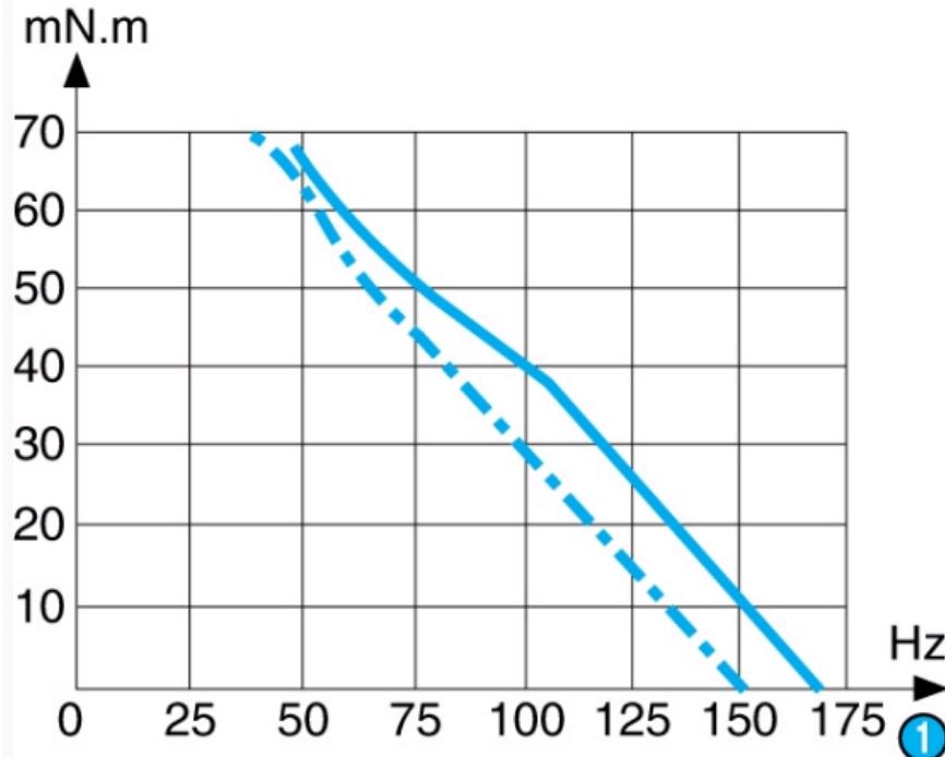
Max. stopping-starting and operating curves at I constant (PBL 3717) for 2 (motor) phases 9 ohms. Holding torque 150 mN.m Current per phase 0.53 A
