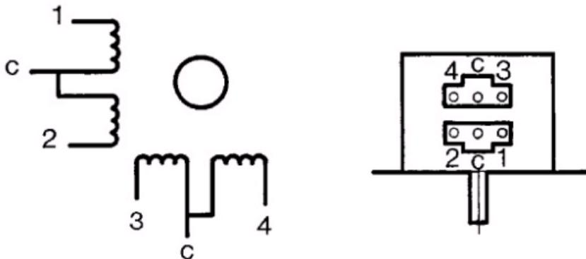
Energisation sequence for clockwise rotation : 2 phases energised (viewed shaft end, front forward) Commons connected to positive.
