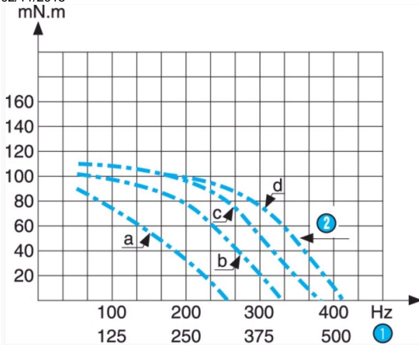
Inertia of measuring chain : 3.4 g.cm<sup>2</sup> a = constant voltage controller with  $R_s$  (resistance in series) = 0 b = constant voltage controller with  $R_s$  (resistance in series) = R motor c = constant voltage controller with  $R_s$  (resistance in series) = 2R motor d = constant voltage controller with  $R_s$  (resistance in series) = 3R motor The measurements are made with full stepping, 2-phases energised.
