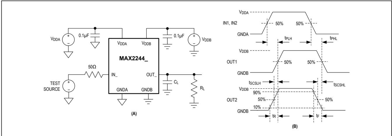
Figure 3. Test Circuit (A) and Timing Diagram (B)
