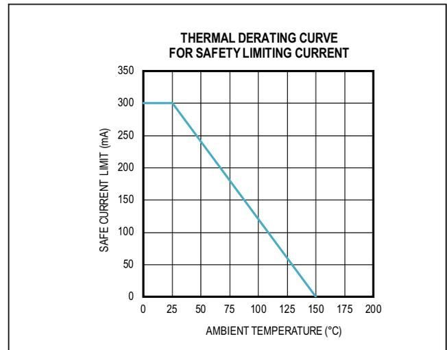
Figure 2. Thermal Derating Curve for Safety Current Limiting
