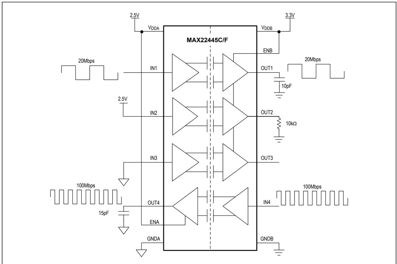
Figure 11. Example Circuit for Supply Current Calculation
