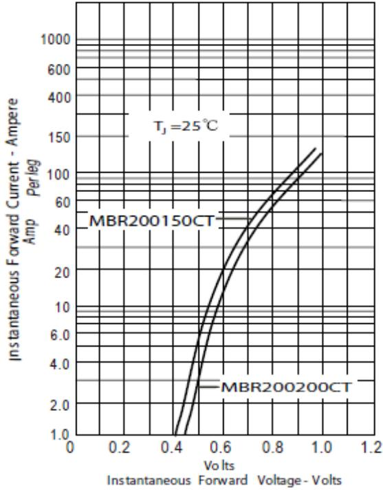
Figure .2- Forward Derating Curve
