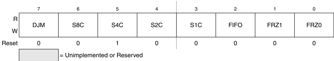
Figure 8-6. ATD Control Register 3 (ATDCTL3)
