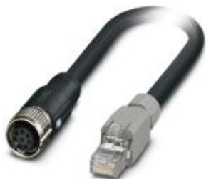
Bus system cable, VARAN, 6-position, SANTOPRENE halogen-free, black RAL 9005, shielded, Plug straight RJ45, on Socket angled M12, cable length: 8 m
