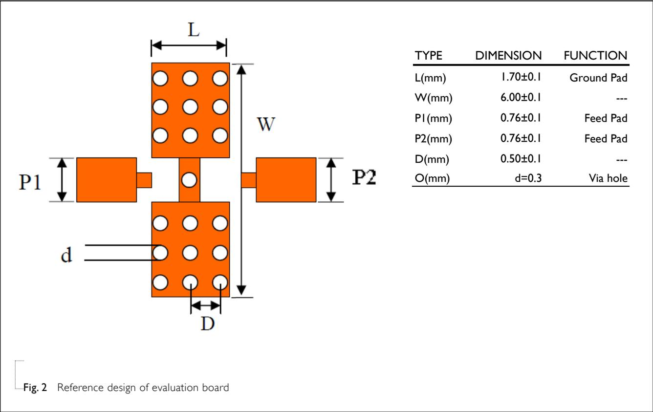
Fig. 2 Reference design of evaluation board
