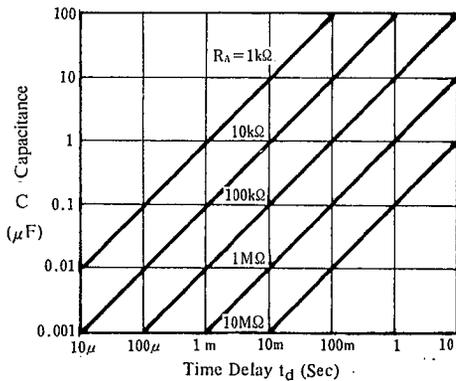
Time Delay vs.  $R_A$ ,  $R_B$  and  $C$
