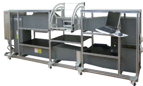
Fig. E: FDK Original Wind Tunnel
