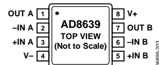
Figure 3. 8-Lead MSOP (RM-8) 8-Lead SOIC_N (R-8)
