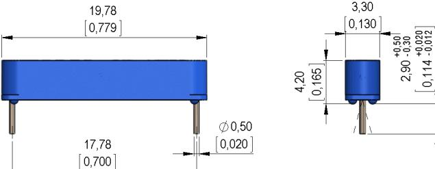
tolerances acc. to DIN ISO 2768-m
