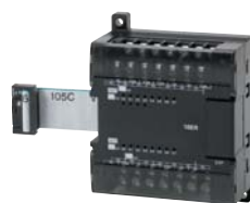
CP1W-16ER ● 16 relay outputs
