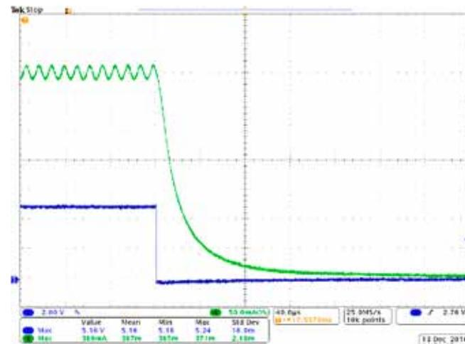
**Fig.7: PWM Dimming at 24V – Fall Time**
