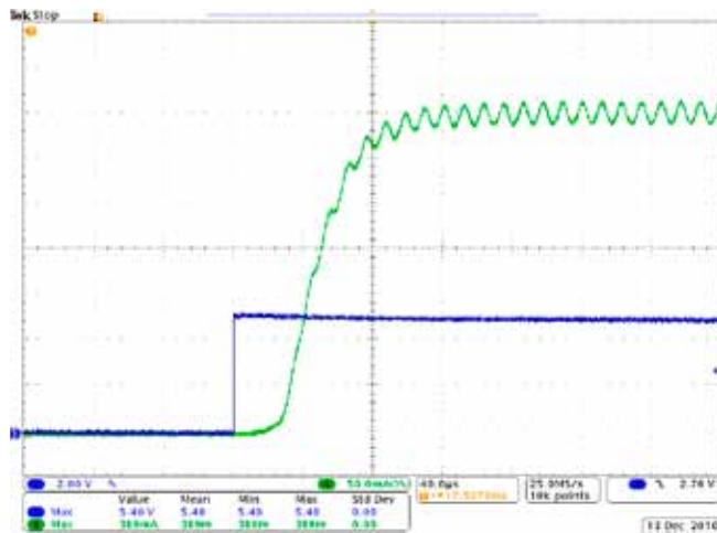
**Fig.6: PWM Dimming at 24V – Rise Time**
