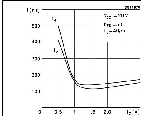
**Figure 9. Switching times resistive load**
