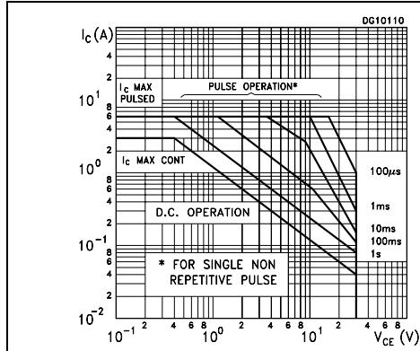
**Figure 3. Derating curve**
