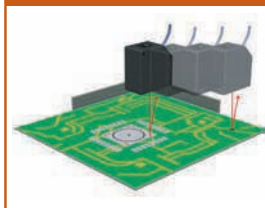
Inspecting Board Heights
