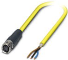
Sensor/Actuator cable, 3-position, PVC, yellow, shielded, Free cable end, on Socket straight M8, Cable length: 10 m
