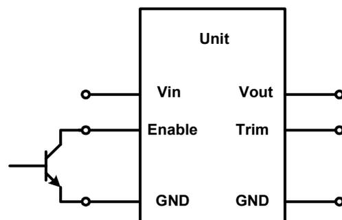
Figure 25: Enable Input drive circuit for D12S300-1 series
