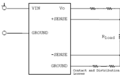
Figure 27 : Circuit configuration for remote sense
