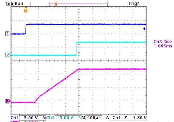
**Figure 16:** Turn on delay time at 12Vin, 2.5V/60A out (1mS/div)
