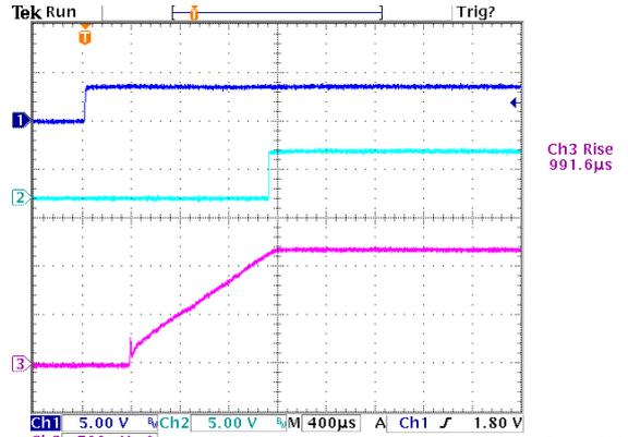
**Figure 14:** Turn on delay time at 12Vin, 1.2V/60A out (1mS/div)
