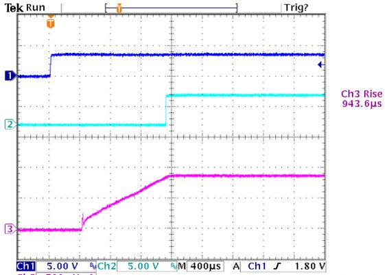
**Figure 13:** Turn on delay time at 12Vin, 0.9V/60A out (1mS/div)
