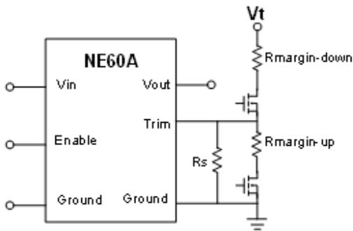
**Figure 29:** Circuit configuration for output voltage margining
