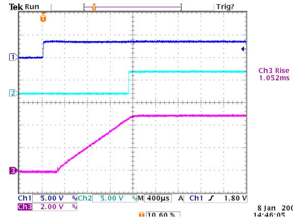
**Figure 18:** Turn on delay time at 12Vin, 5.0V/60A out (1mS/div)
