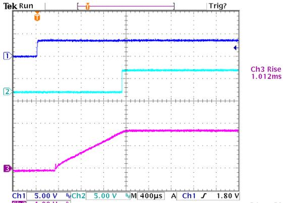
**Figure 15:** Turn on delay time at 12Vin, 1.8V/60A out (1mS/div)
