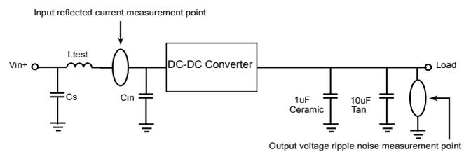
$C_s=330\mu\text{F OS-CON cap x 1}$ ,  $L_{\text{test}}=1\mu\text{H}$ ,  $C_{\text{in}}=330\mu\text{F OS-CON cap x 1}$
