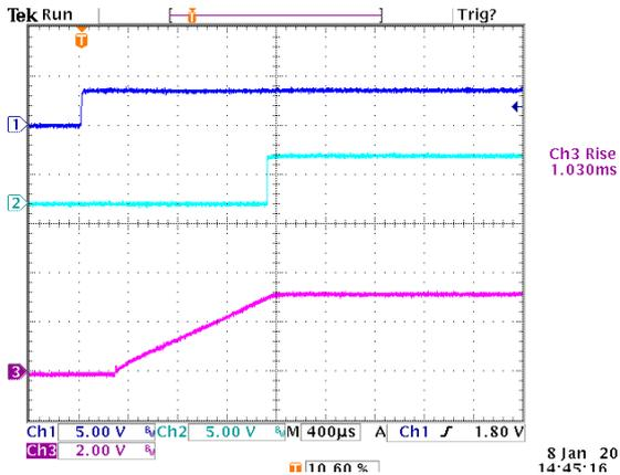
**Figure 17:** Turn on delay time at 12Vin, 3.3V/60A out (1mS/div)
