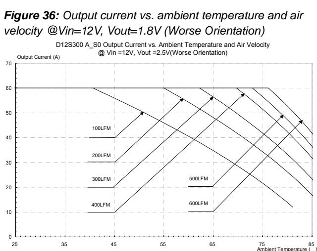
**Figure 37:** Output current vs. ambient temperature and air velocity @ Vin=12V, Vout=2.5V (Worse Orientation)
