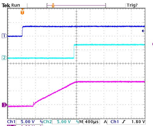
**Figure 15:** Turn on delay time at 12Vin, 1.8V/60A out (1mS/div)
