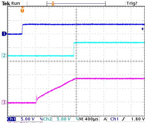
**Figure 13:** Turn on delay time at 12Vin, 0.9V/60A out (1mS/div)
