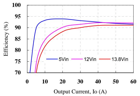
**Figure 4:** Converter efficiency vs. output current
