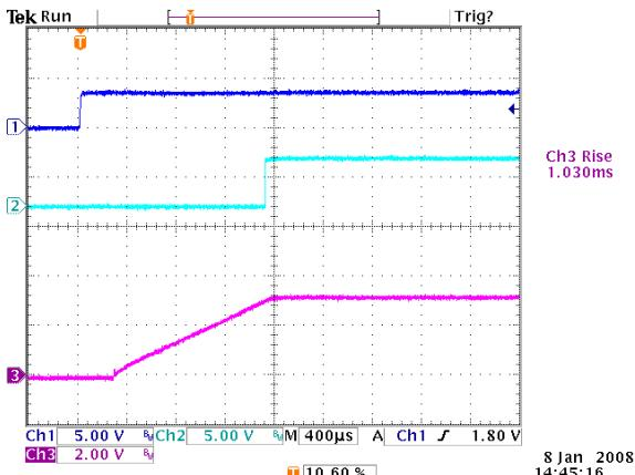
**Figure 17:** Turn on delay time at 12Vin, 3.3V/60A out (1mS/div)
