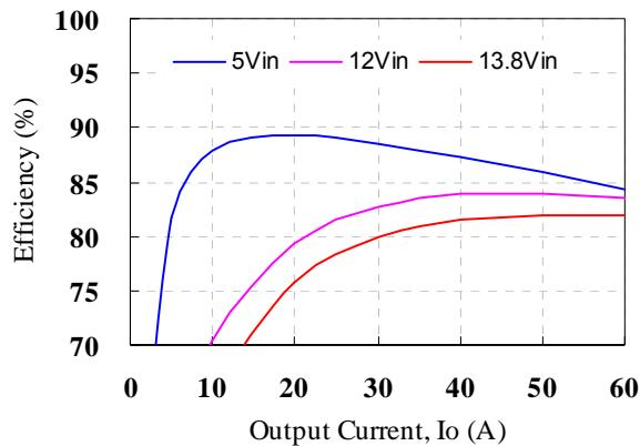
**Figure 1:** Converter efficiency vs. output current
