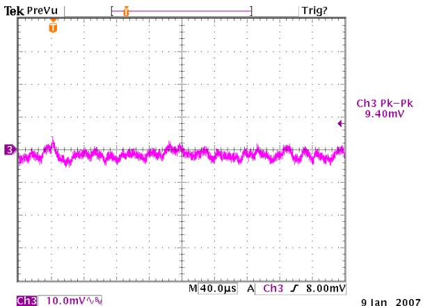
**Figure 9:** Output ripple & noise at 12Vin, 1.8V/60A out
