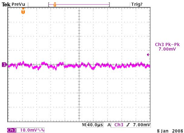
**Figure 7:** Output ripple & noise at 12Vin, 0.9V/60A out
