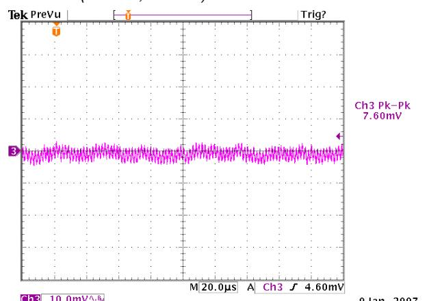
**Figure 12:** Output ripple & noise at 12Vin, 5.0V/60A out
