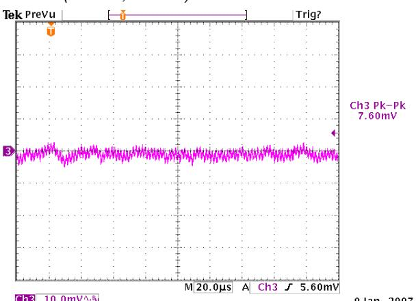
**Figure 11:** Output ripple & noise at 12Vin, 3.3V/60A out
