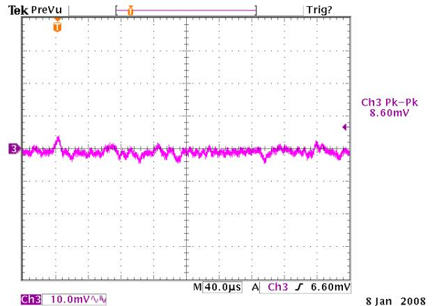
**Figure 8:** Output ripple & noise at 12Vin, 1.2V/60A out
