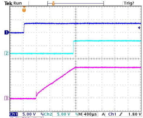
**Figure 14:** Turn on delay time at 12Vin, 1.2V/60A out (1mS/div)
