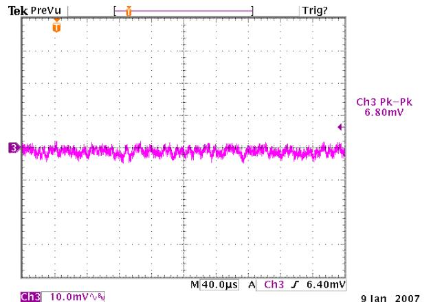
**Figure 10:** Output ripple & noise at 12Vin, 2.5V/60A out
