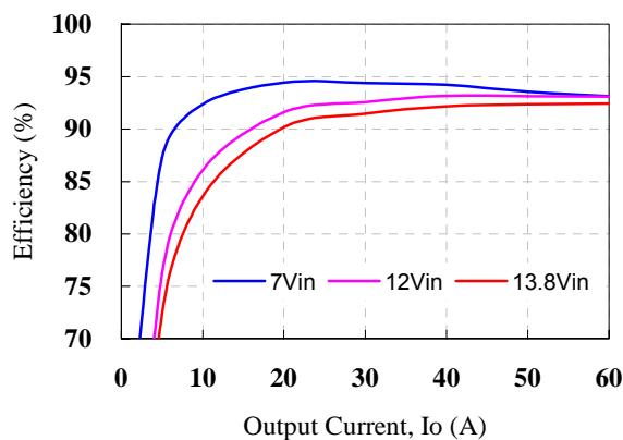
**Figure 5:** Converter efficiency vs. output current
