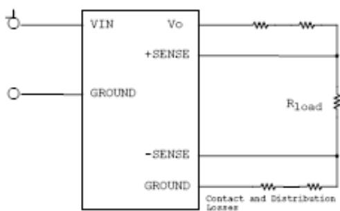
**Figure 27 :** Circuit configuration for remote sense
