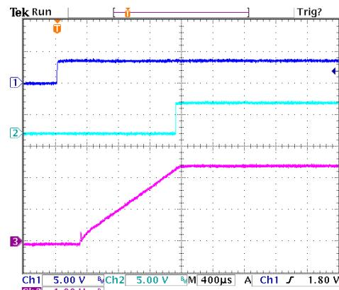
**Figure 16:** Turn on delay time at 12Vin, 2.5V/60A out (1mS/div)
