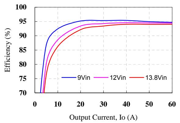
**Figure 6:** Converter efficiency vs. output current
