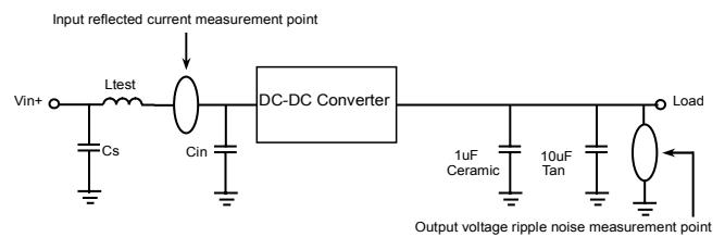
$C_s = 330\mu\text{F}$  OS-CON cap x 1,  $L_{\text{test}} = 1\mu\text{H}$ ,  $C_{\text{in}} = 330\mu\text{F}$  OS-CON cap x 1
