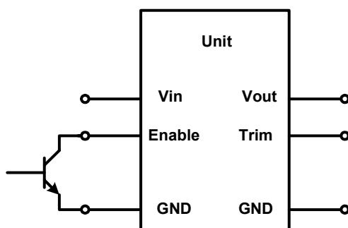
Figure 25: Enable Input drive circuit for D12S300-1 series
