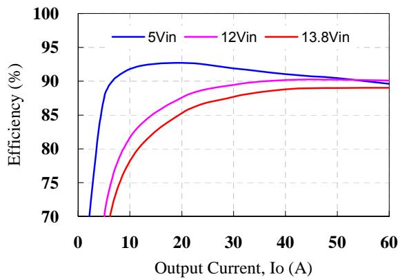
**Figure 3:** Converter efficiency vs. output current
