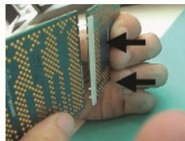
Figure 2 – 2<sup>nd</sup> SchmartBOARD™ connected to the 1<sup>st</sup> SchmartBOARD™ via a Schmart mechanical bridge
