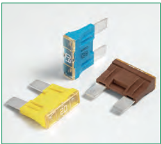
TOE MAXI® style 58V Slo-Blo® Automotive Copper Blade Fuse Amps (A): 20, 30, 40, 50, 60, 70
