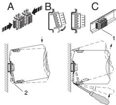
Figure 4 Assembly and removal
