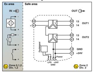
Figure 1 Basic circuit diagram with connection terminal
