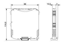
Figure 3 Dimensions (in mm)
