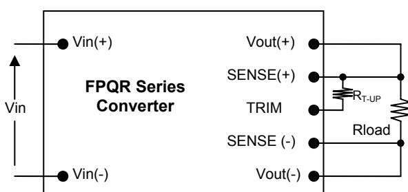
Fig. C: Configuration for trimming output voltage up
