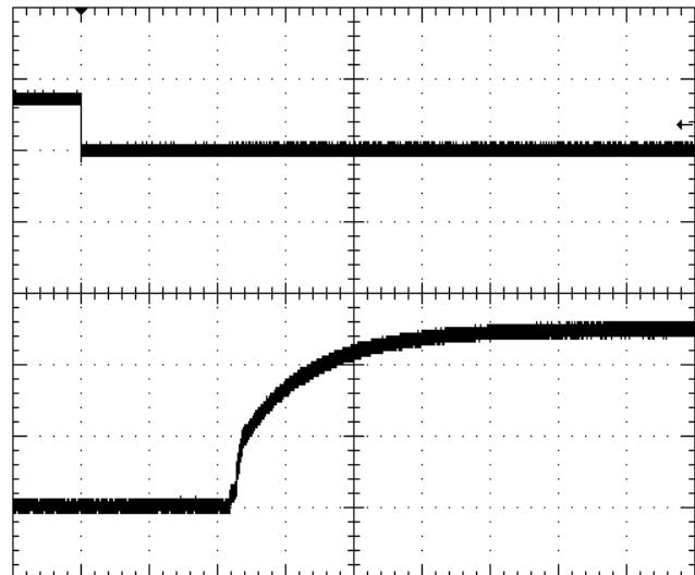
**Fig-5:** Turn-on transient at full rated load current (resistive) plus  $20,000\mu\text{F}$  at  $V_{in}=48\text{V}$ , triggered via ON/OFF pin. Top trace: ON/OFF signal (5V/div). Bottom trace: output voltage (2V/div). Time scale: 10ms/div
