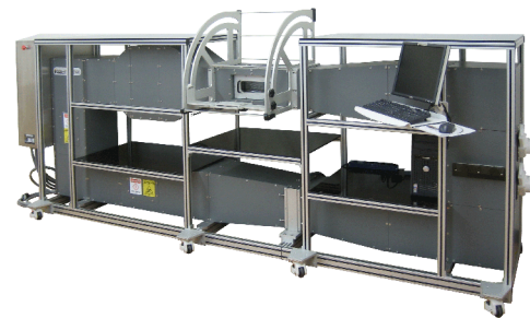
Fig. E: FDK Original Wind Tunnel
