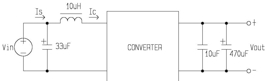
**Fig-8:** Test Set-up for measuring input reflected ripple current.
