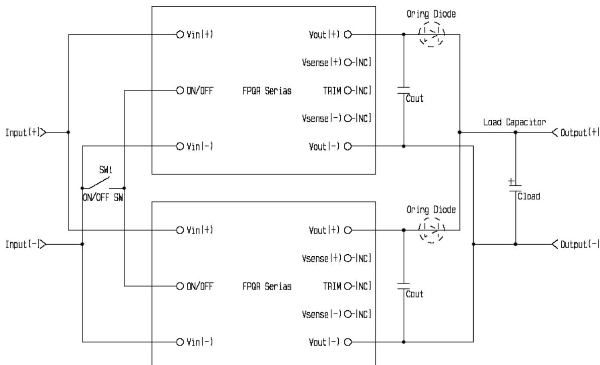
Sch-1 : Circuit for using the parallel option
