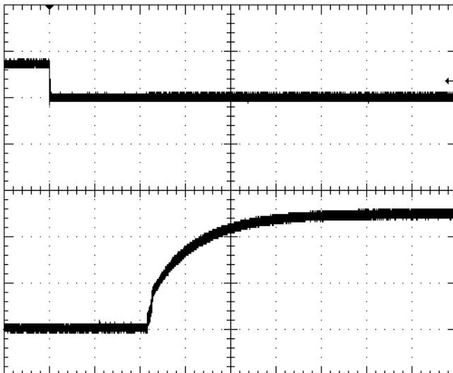
**Fig-4:** Turn-on transient at full rated load current (resistive) with  $10\mu\text{F}$  tantalum +  $1\mu\text{F}$  ceramic capacitor at  $V_{in}=48\text{V}$ , triggered via ON/OFF pin. Top trace: ON/OFF signal (5V/div). Bottom trace: output voltage (2V/div). Time scale: 2ms/div
