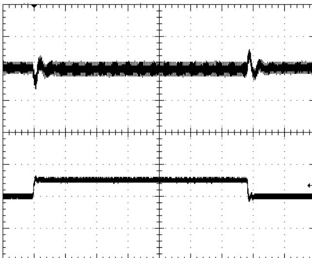
**Fig-6:** Output voltage response to load current step-change (20A-30A-20A) at  $V_{in}=48\text{V}$ . Top trace: Output voltage (200mV/div). Bottom trace: load current (20A/div). Current slew rate:  $5\text{A}/\mu\text{s}$ .  $C_o=470\mu\text{F}$  Low Z EL-con +  $10\mu\text{F}$  ceramic. Time scale:  $200\mu\text{s}/\text{div}$
