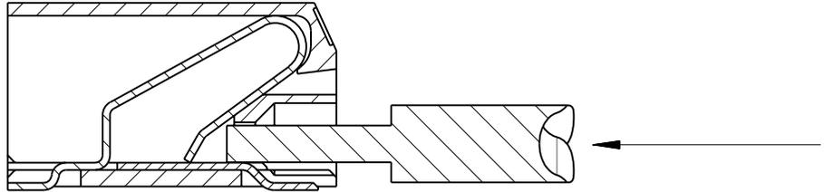
PUSH WIRE INTO HOLE IN FRONT OF CONNECTOR.
