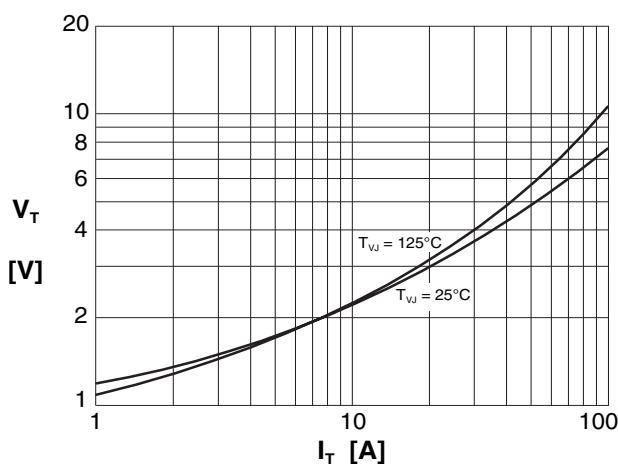
Fig. 3 On-state voltage
