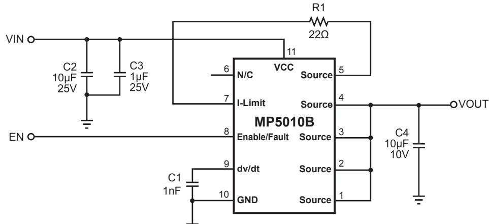
Figure 4: Typical Application Schematic with Kelvin Current Sensing
