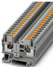
Feed-through terminal block, Connection method: Push-in connection, Cross section: 0.5 mm 2 - 10 mm 2 , AWG: 20 - 8, Width: 8.2 mm, Height: 42.2 mm, Color: orange, Mounting type: NS 35/7,5, NS 35/15
