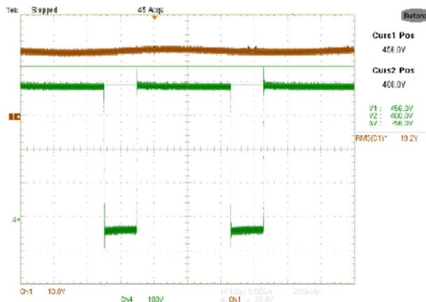
**Figure 13. Waveforms of  $V_{DS}$  of Q2 at  $I_L=20A$
