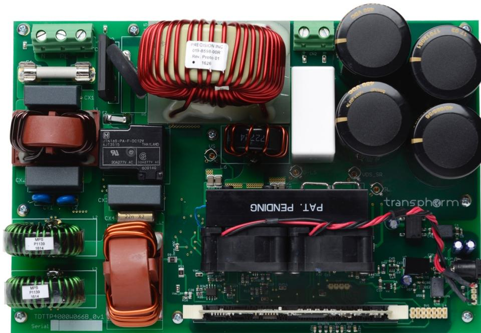
Figure 1. TDTP4000W066B\_0v1 4kW totem-pole PFC evaluation board
