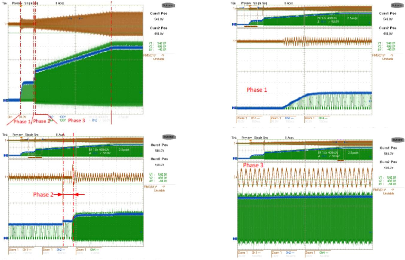
Figure 10. Start-up of the bridgeless totem-pole PFC with 1.2kW load
