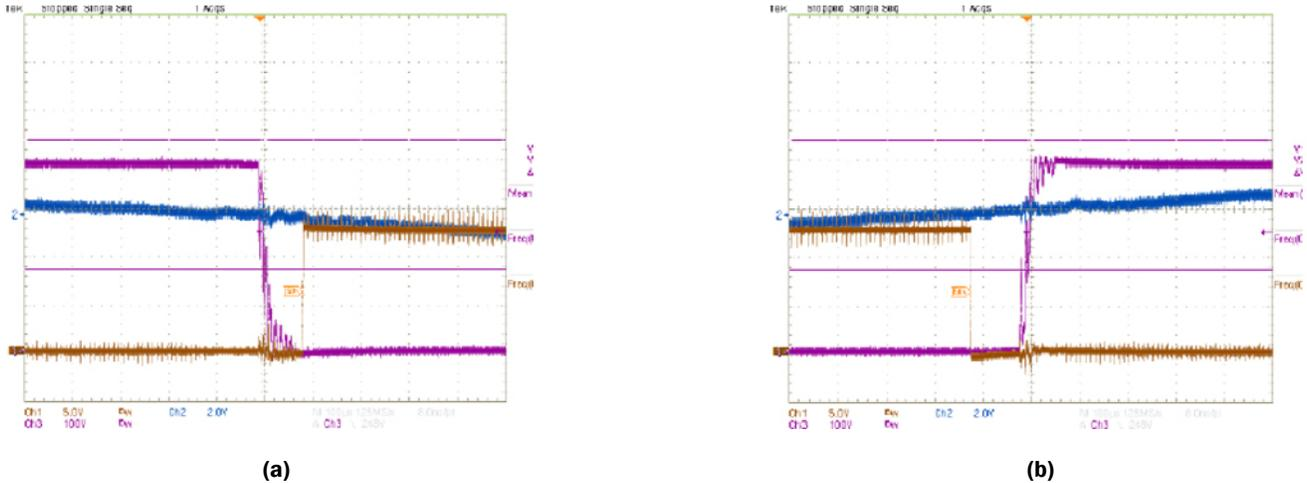
**Figure 14. Zero-crossing transitional waveforms (a) from negative to positive half-cycle and (b) from positive to negative half-cycle
