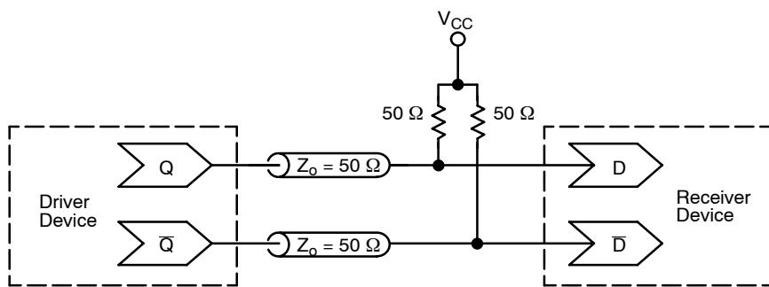
**Figure 9. Typical Termination for Output Driver and Device Evaluation
