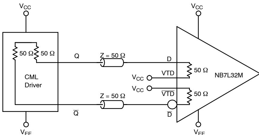
**Figure 15. CML to NB7L32M Interface**
