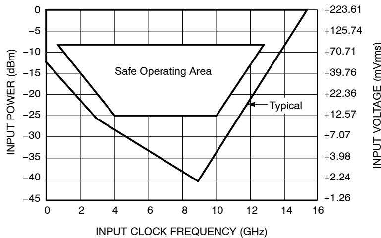
**Figure 3. Input Signal Amplitude vs Input Clock Frequency (All Temperatures and Power Supplies; Guaranteed Output Amplitude of at Least  $V_{OUTPP} = 160\text{ mV}$ )**
