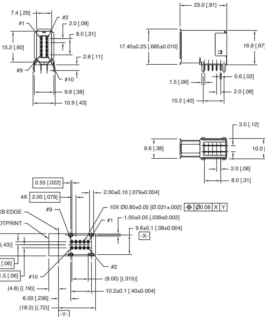
Recommended PCB hole mounting pattern
