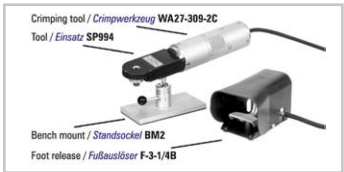
Crimping tool / Crimpwerkzeug WA27-309-2C Tool / Einsatz SP994 Bench mount / Standsoclel / BM2 Foot release / Fußauslöser F-3-1/4B Tool order number: WA27-309-2C with foot release BM-2 (bench mount) SP994 (positioner) TP1071-1, TP1072-1 (positioner)
