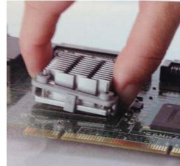
**STEP 1:** Center heat Sink onto BGA. Tilt and hook one side of the clip under the BGA chip.
