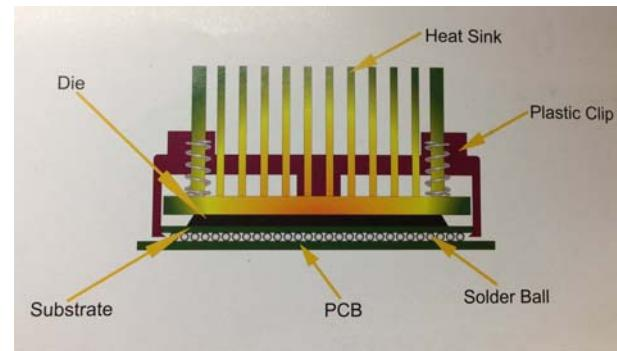
Wakefield-Vette heat sink assembles onto chip set using the space that is between the PCB and the substrate of the solder balls. The solder balls provide a minimal gap of .5mm to .7mm. Attachment feature is below a .4mm thickness. The clipping system will not interfere or damage chip. Contact area is the edge of chip.
