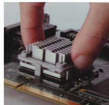
**STEP 3:** Make sure the stop pin is not on top of the chip set. Installation Done!
