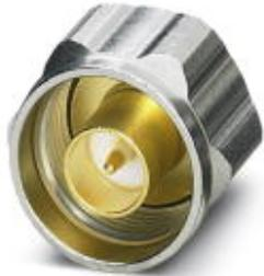
A termination resistor must be screwed on at the end of the leaky wave conductor which does not contain any wireless part. It guarantees an antenna cable termination with the correct impedance and is important for every wireless installation.
