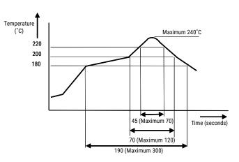
Note: Temperature profile shows printed circuit board surface temperature on the relay terminal portion. Please consult KEMET if you wish to use a temperature profile other than above.
