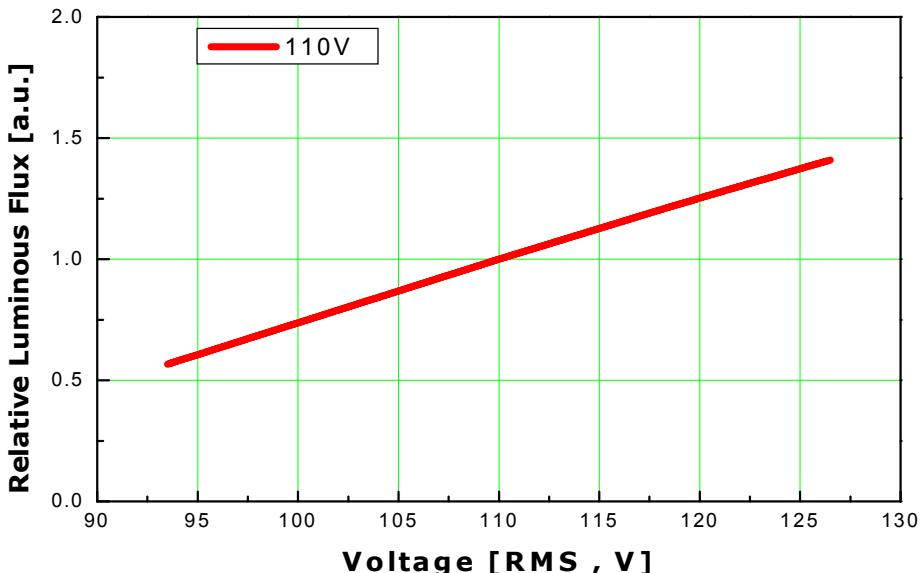
**Voltage – Relative flux characteristics, Ta=25°C**
