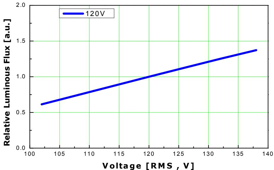
**Voltage – Relative flux characteristics, Ta=25°C****4. AX3220 with external resistor @220V**
