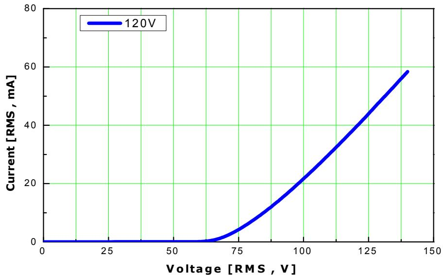
**Current – Voltage characteristics, Ta=25°C****4. AX3220 with external resistor @220V**
