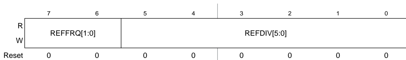
Figure 7-4. S12XECRG Reference Divider Register (REFDV)
