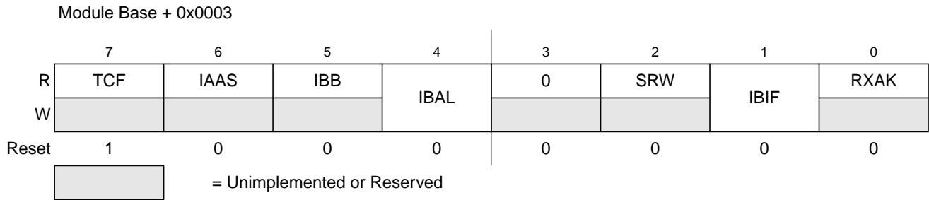
Figure 12-7. IIC Bus Status Register (IBSR)
