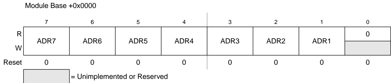
Figure 12-3. IIC Bus Address Register (IBAD)
