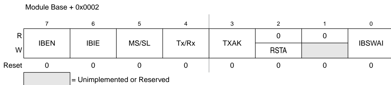
Figure 12-6. IIC Bus Control Register (IBCR)
