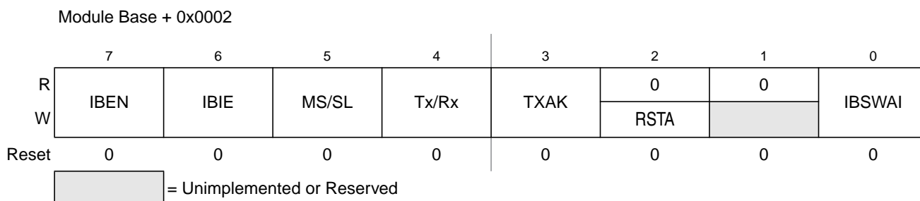
Figure 12-6. IIC Bus Control Register (IBCR)
