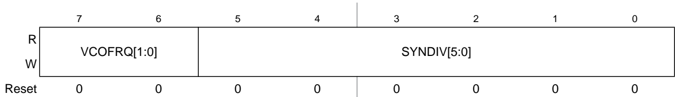
Figure 7-3. S12XECRG Synthesizer Register (SYNR)
