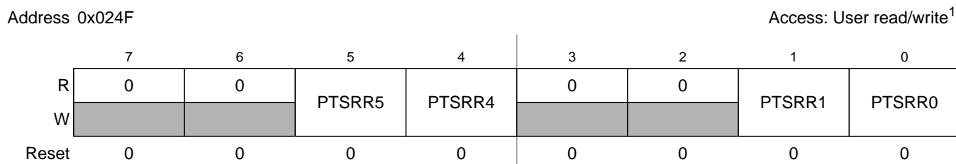
Figure 2-27. Port S Routing Register (PTSRR)
