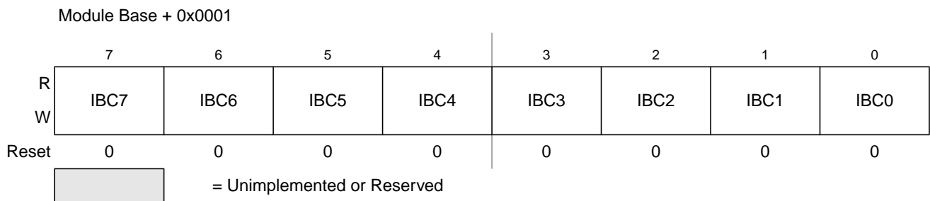
Figure 12-4. IIC Bus Frequency Divider Register (IBFD)
