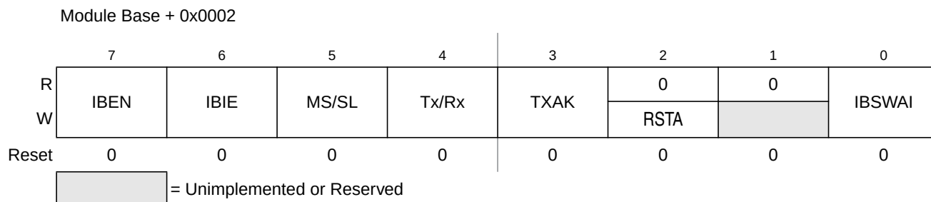
Figure 12-6. IIC Bus Control Register (IBCR)
