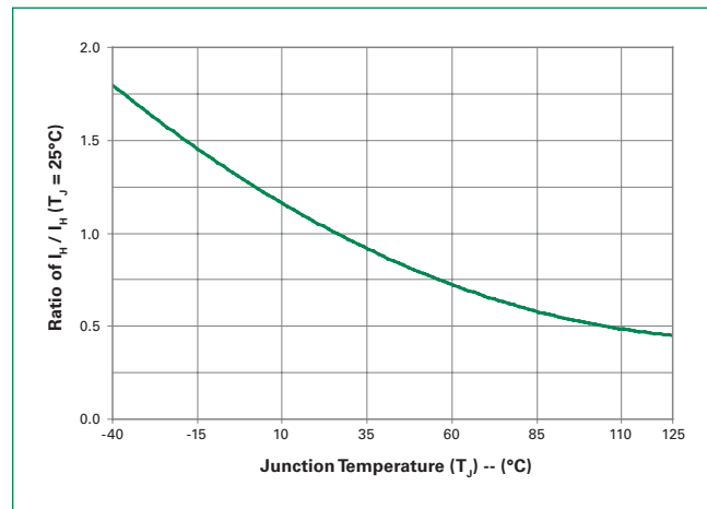
Figure 4: Normalized DC Holding Current vs. Junction Temperature
