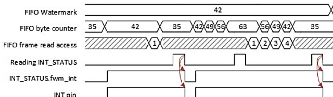
FIFO watermark interrupt, latched, with reads from FIFO
