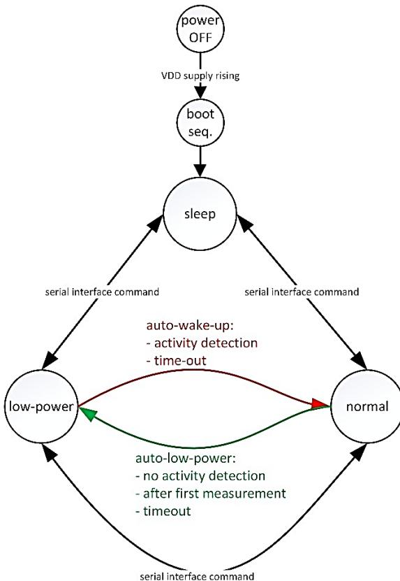
In **sleep mode**, current consumption is 200nA, and data conversions are stopped as well as sensortime functionality.
