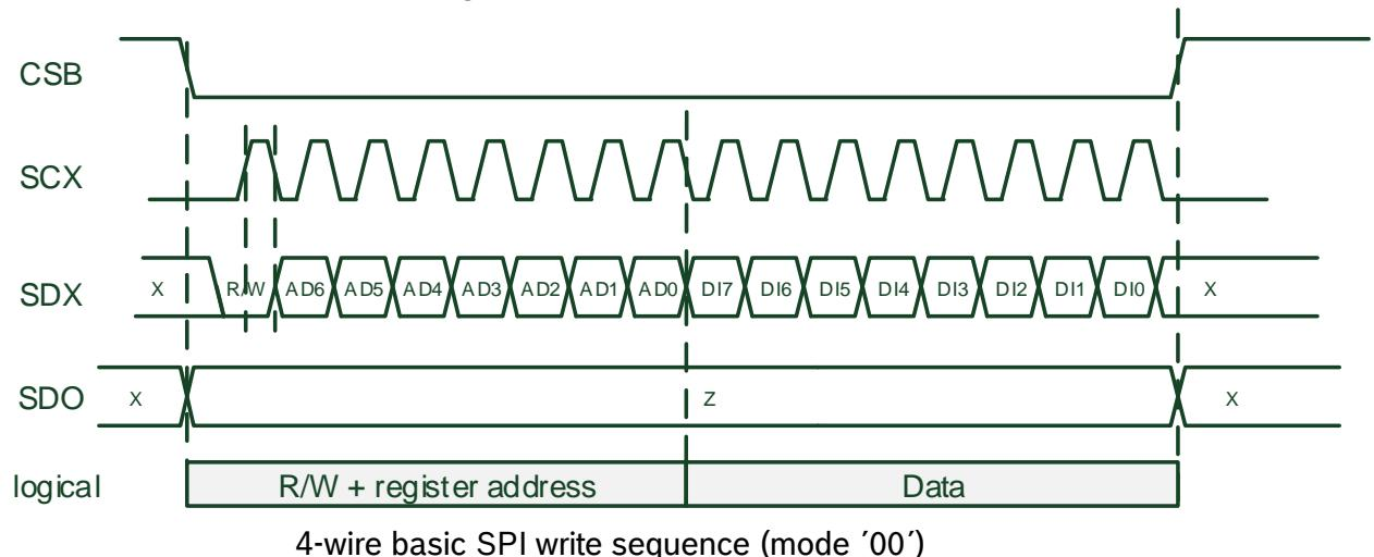
Multiple write operations are possible by keeping CSB low and continuing the data transfer. Every data must be preceded by R/W flag and address, there is no address auto-increment like in burst read mode. The principle of multiple write is shown in figure below:
