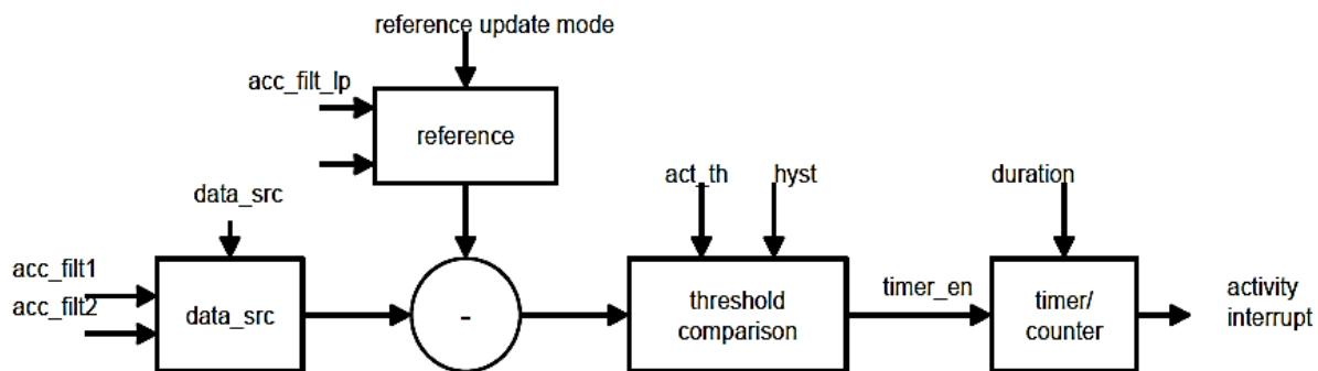
The data rate for the filter output must be 100Hz. Using acc\_filt2 is recommended. In this case acc\_filt1 can be used independently from the interrupt engine for the data output registers and the FIFO.
