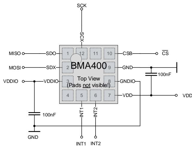
It is recommended to use 100nF decoupling capacitors at pin 3 (VDDIO) and pin 7 (VDD).
