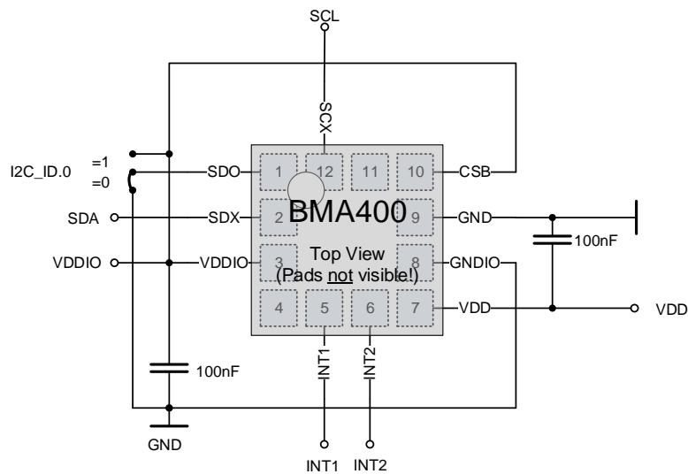
It is recommended to use 100nF decoupling capacitors at pin 3 (VDDIO) and pin 7 (VDD).
