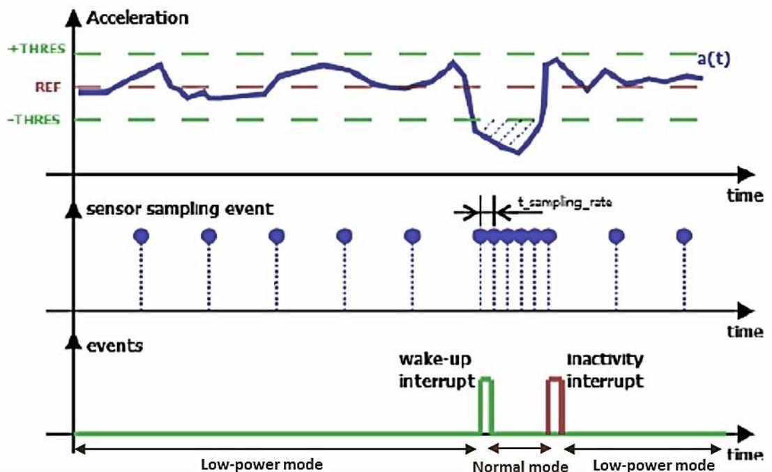
Wake-up interrupts can be used latched and non-latched (see chapter 0). Latched and non-latched behavior is shown below.
