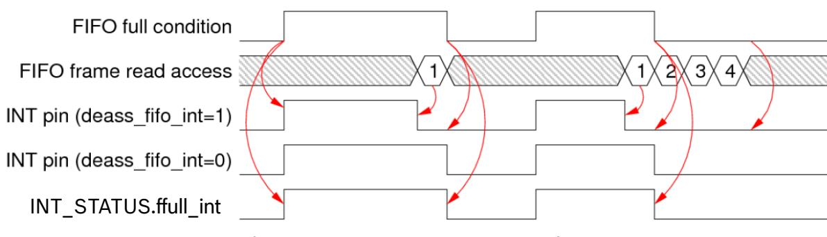
FIFO full interrupt, non-latched, with reads from FIFO
