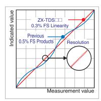
The long-stroke ZX-TDS04T□ (4-mm measurement range) achieves high-precision measurement with the industry's top class of resolution (0.1 µm) and linearity of 0.3 FS max.
