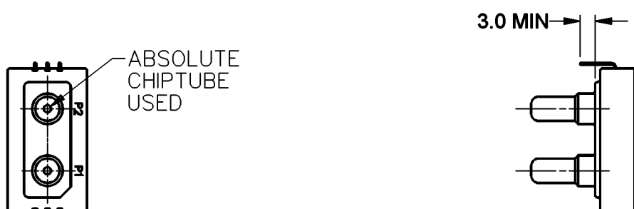
TYPE "A" (ABSOLUTE) MOUNTING TYPE = "P"
