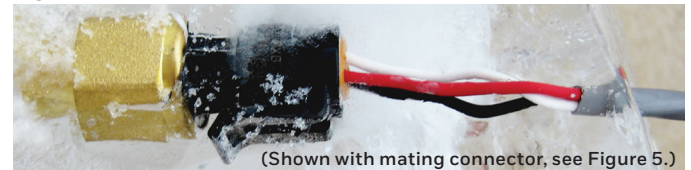
Figure 2. PX3 Series External Freeze/Thaw Resistance
