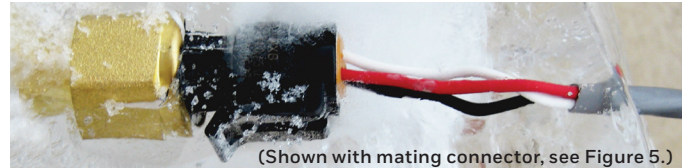
Figure 2. PX3 Series External Freeze/Thaw Resistance
