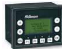
Remote LCD screen / keypad + 4 function buttons + 4 LEDs
