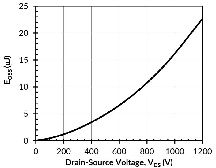
Figure 12. Typical stored energy in  $C_{\text{OSS}}$  at  $V_{\text{GS}} = 0\text{V}$
