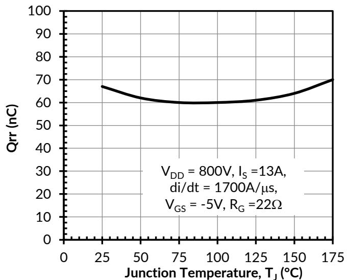
Figure 22. Reverse recovery charge  $Q_{rr}$  vs. junction temperature
