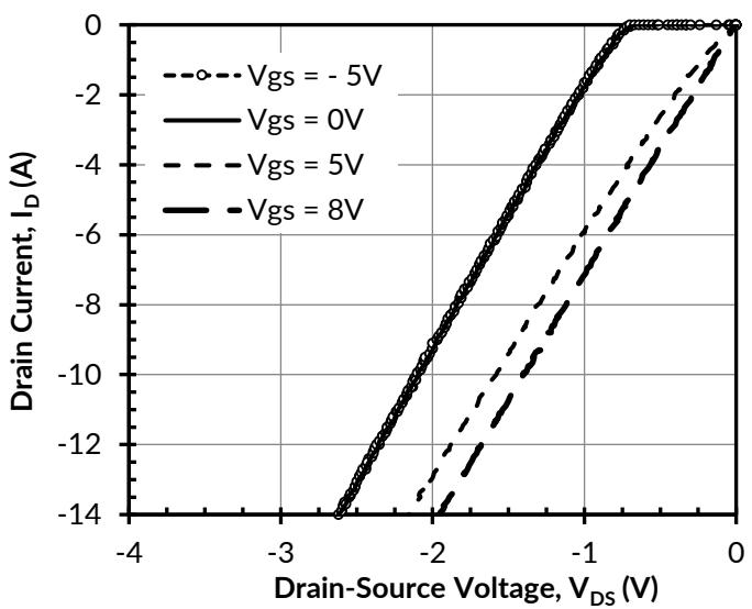
Figure 10. 3rd quadrant characteristics at  $T_J = 25^\circ\text{C}$
