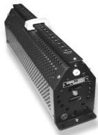
These variable rheostats are produced using constantan (CuNi44) wire, wound onto ceramic formers, with insulated wire to give mechanical stability and good heat dissipation.
