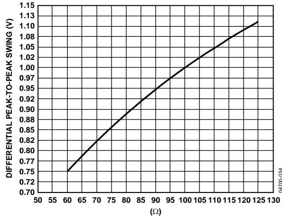
Figure 34. Peak-to-Peak DAC Output Swing vs. Swing Scaling Resistor R3 (R1 = R2 = 50 \Omega )
